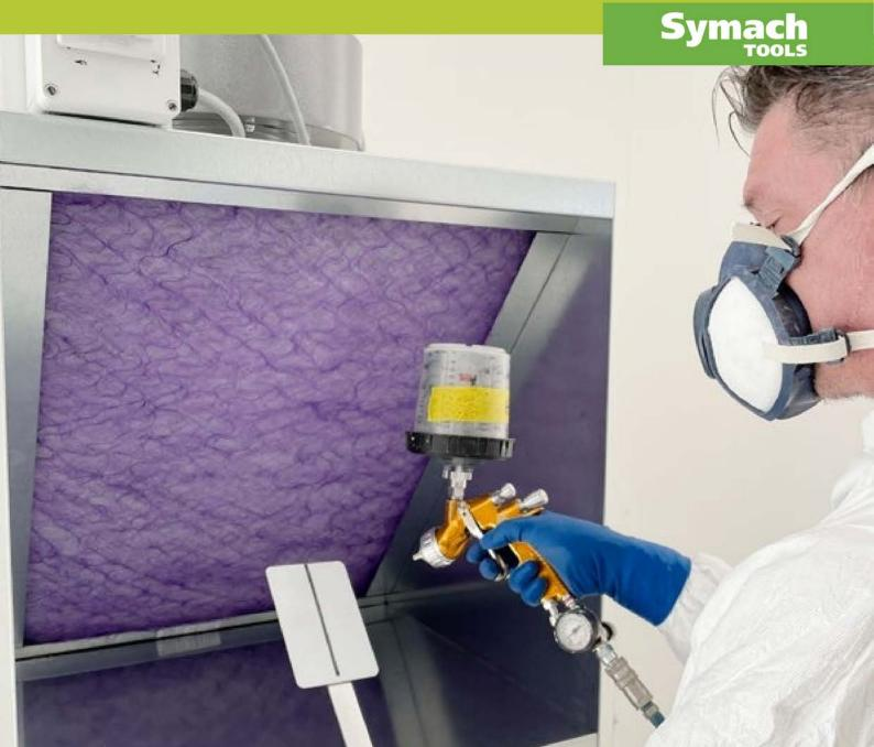
The mini booth **allows you to paint color sample cards outside of your spraybooth.** Thanks to its highly efficient extraction fan, it avoids spreading paint vapors and fumes into the environment. Its high capacity filter is easy to replace. It's compact and can be placed anywhere in the body shop. Made of non-corrosive and solvent resistant materials, it's solid and easy to install and use, requiring minimum maintenance.
